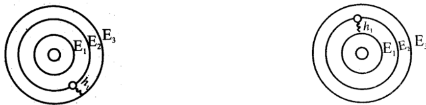
Fig. 3.11 : Absorption and emission of photon causes the electron to change its energy level.
