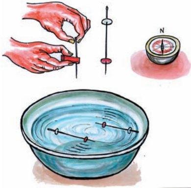
Fig-2: Making needle magnets and floating them in a bowl of water.
