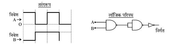
Using the input A and B, waveforms, draw the output waveform of the given logic circuit. Identify the logic gate obtained. Write its truth table.
